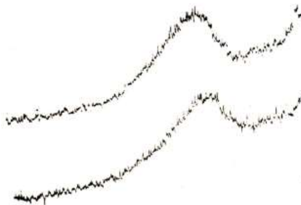
Fig.4 Perlite X-ray diffraction patterns. a) Upper –raw perlite; b) lower – perlite sintered at 900°C
